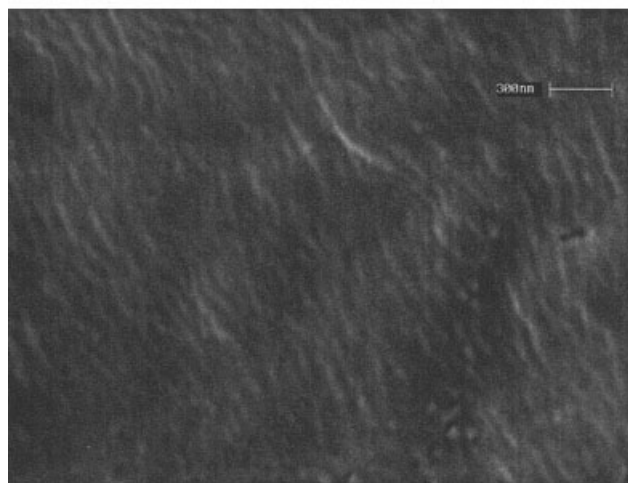
Figure 6 SEM images of UHMWPE tapes made from (a) 30C_15P and (b) 90C_40P UHMWPE powders. The tapes were etched with a 7\text{K}_2\text{CrO}_7 \cdot 150\text{H}_2\text{SO}_4 \cdot 12\text{H}_2\text{O} solution for 1 h.
